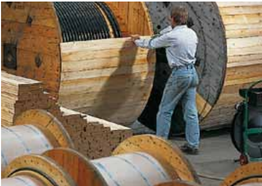
The tube bundle is wound onto wooden reels.
